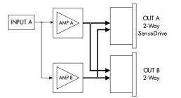
D12 Input/Output routing 2-Way Active mode
