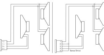
NLT4 F and EP5 connector wiring
